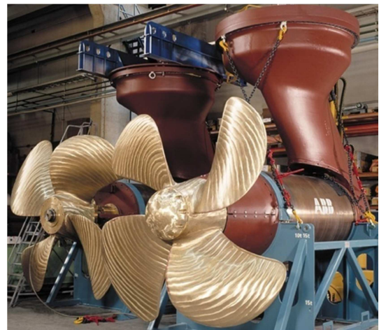
Figure 17. ABB Azipod propulsion systems and Azipods (2 units) fitted on Oasis-class cruise ship [111].
